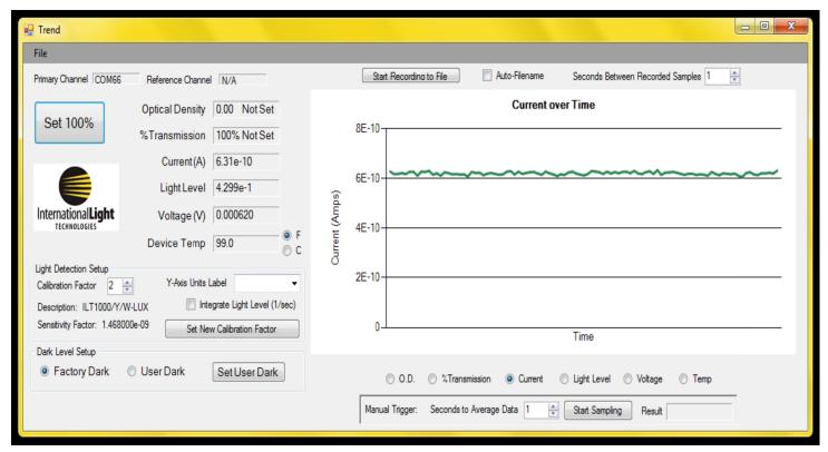
**1. Trend** is a **single unit**, graphical interface program which allows easy monitoring of changes in data. Users may select to run single or multiple copies of Trend.
