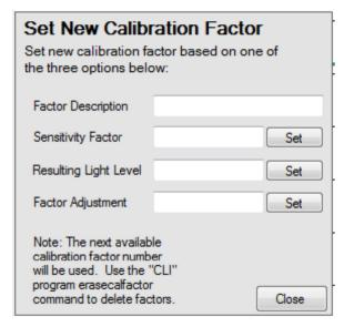
Resulting Light Level: SELF CALIBRATION. This process allows the end user to create a calibration factor which will force the meter to read a known value. Example: You have a calibrated light source with a known output in lux. Enter the lux value ie 100. The software will calculate what sensitivity factor would be needed to acquire a reading of 100 and will store a new calibration factor in the next available channel. click "Set" and "Close" when done.
