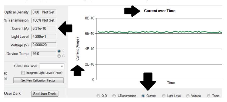
Trend allows the user to select which measurements (such as light level or voltage) are viewed in the display graph by clicking on the appropriate radio button shown just below the graph.
