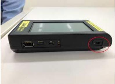
A close-up view of the bottom of the ILT2400 host, showing various ports (USB, FireWire) and a power switch. The power switch is circled in red.          | <p>3.把 ILT2400 开关打开,准备进行量测</p>                 |
