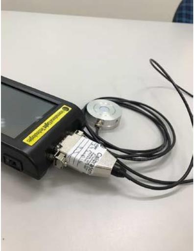
A close-up view of the black cable being plugged into the back of the ILT2400 host. The cable has a white label with 'Cable 800' printed on it.            | <p>2.使用时,先把 ILT2400（主机） 与 Detector（探头）连接起来</p> |
