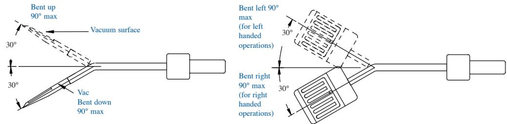
To order a longer tube length, up to 8" (203.20mm) long, add a "-XL" to the Wafer Tip part number where "X" is the total length of the tube desired. To specify an angle to be included on the tube, add a "-YD" to the part number where "Y" is the angle that is required.
