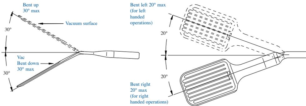
Molded Wafer Tips VMWT-A, VMWT-B and VMWT-C are available with a 10°, 20° or 30° bend in the up or down direction as shown in the left drawing above. To order a tip with the up or down bend, add the angle plus a "U" for up or a "D" for down to the part number. *EXAMPLE: Part number VMWT-A20D is a VMWT-A Wafer Tip with a 20 degree bend in the down direction. Custom angles are available upon request. Pricing is as above.*
