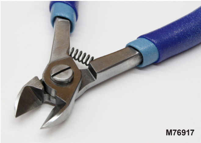
Large Oval Full Flush Cutter Designed for flush lateral cutting of heavy duty materials such as stainless steel and Nitinol up to .035”.
